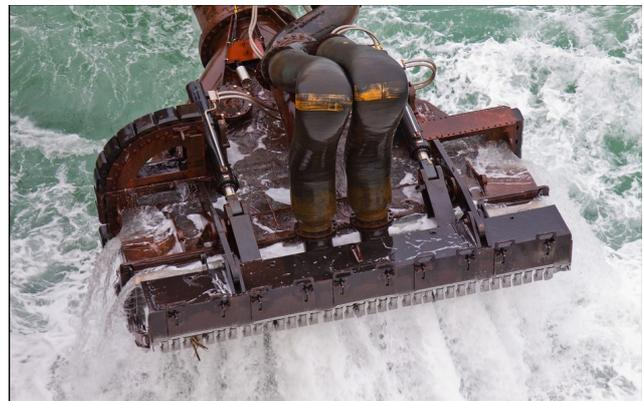
*Frequently applied full ceramic piston rod coatings to dredging equipment is often not sufficiently impact resistant. Apart from the outstanding corrosion protection, Lunac 2+ duplex proved to resist most stone chips even without any cracking*
