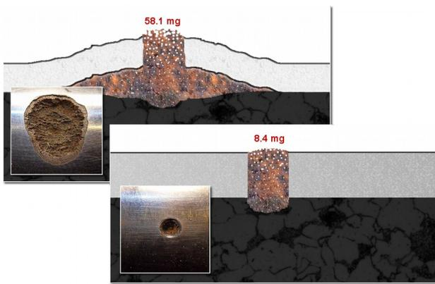
*Corrosion behaviour after 8 days acidified salt water test in two 3.0 mm pre drilled holes. The first graphic pair shows the reaction of a duplex hard chromium coating and the second graphic pair the reaction of a Lunac 2+ duplex coating. The Lunac 2+ duplex coating reduces the total amount of corrosion (red numbers) and highly inhibits subsurface corrosion.*
