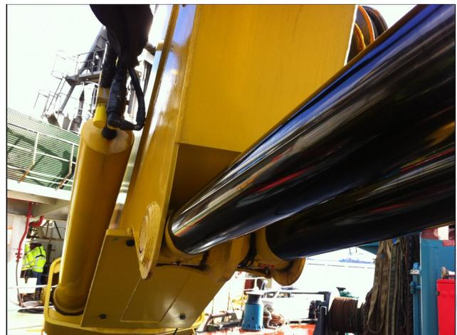
*Lunac 2+ duplex applied to hydraulic piston rods, dealing with very hard (mechanical and corrosive) conditions after several years. All preceding coatings failed within 2 years at this spot. These piston rods clearly present the Lunac 2+ dark grey appearance that typically comes along with the Lunac 2+ surface under these harsh conditions.*
