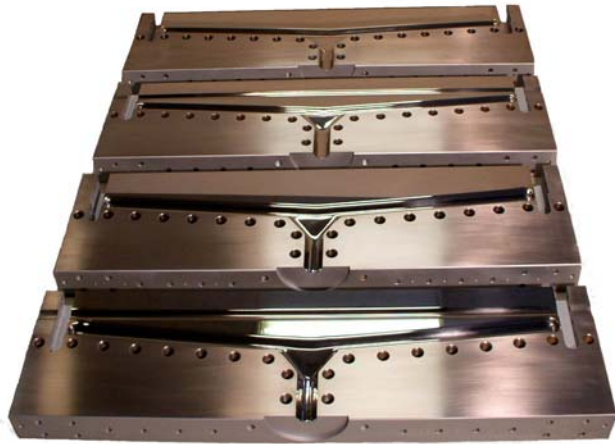
Figure 3. Flat dye extrusion parts completely coated with 0,002" Lamac 1. The reduced friction together with the anti striping effect is striking. This manufacturer utilizes the high corrosion resistance together with the very closed Lamac 1 structure very efficiently. Instead of (partially) corrosion resistant steel, this manufacturer applies a low grade steel. This steel is much easier to machine as well. All necessary surface features are delivered by the Lamac 1 coating. This concept has irrefutable proven to be superior to a non coated chromiumsteel flat dye after 3 years application (See figure 4). The possible bending of the lip has to be limited because of the brittleness of Lamac 1 (0,11% elongation until breakage).
