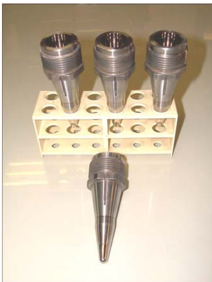
Injection nozzles for DVD production treated with Lunac 1 on the inner surface. If only these end parts of an injection system are treated, a reject percentage due to black spots is generally reduced by 45%. Up until the present time only the complete Lunac 1 treated injection system solves the black spots problem completely. The end opening is only 0.07" wide (measured over a length of 0.16") and completely plated.
