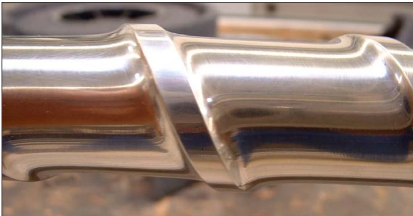
Picture 7. Lunac 1 replacement for Hastelloy CA. 1.4" screw after 5 weeks in a PFA fluoroplastic environment. Not any corrosion effect has been detected. Basic material: PH 17-4.
