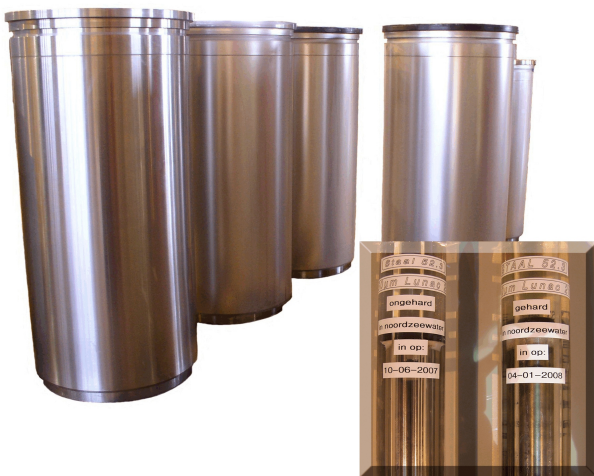
Picture 1: Hydraulic cylinder for offshore-industry, (600 metric tons) coated with Lunac 2+. The coating thickness on the outside is generally 55-70 \mu\text{m} and 10 \mu\text{m} on the inside. The unparalleled high corrosion protection is mainly caused by the entirely closed structure. The high wear- and scratch resistance is caused by the high hardness (harder than quartz sand) and toughness of this material. The continuing metal lattice from the substrate up to the coating causes the welding quality bond. Especially the high reliability of the Lunac 2+ coating is frequently mentioned by the applicants. The insert displays a long term seawater corrosion test. Two Steel 52.3 rods are coated with 50 \mu\text{m} Lunac 2+ since 10-08-2007
